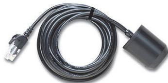
The photosynthetically active radiation (PAR) smart sensor is designed to work with HOBO<sup>®</sup> stations. The smart sensor has a plug-in modular connector that allows it to be added easily to a station. All calibration parameters are stored inside the smart sensor, which automatically communicates configuration information to the logger without any programming, calibration, or extensive user setup.
