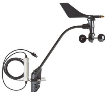
The Davis Wind Speed and Direction smart sensor is designed to work with HOBO® stations. The smart sensor has a plug-in modular connector that allows it to be added easily to a HOBO station. All sensor parameters are stored inside the smart sensor, which automatically communicates configuration information to the logger without the need for any programming or extensive setup. **Note:** This sensor has been modified to work with Onset station loggers only.
